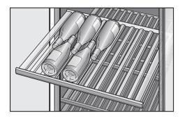
The wooden shelves are on telescopic runners which can be pulled out to make it easier to store and remove bottles.
